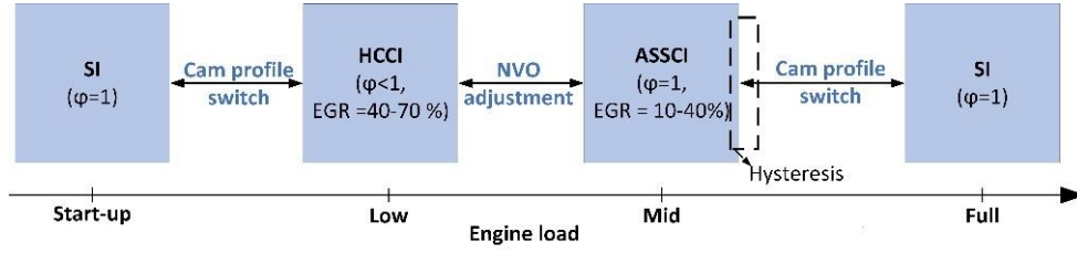
Figure 2.21: SI-HCCI-ASSCI-SI multi-mode engine and the corresponding combustion characteristics [14]
